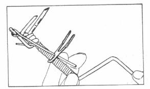
To set trap hold trap handle in 4. right hand, and catch spring latch with left thumb and place two fingers under the spring (as shown in the drawing). Hold firm cranking the trap handle to the right until the spring latch meets the trap handle and is latched to the trap handle.
