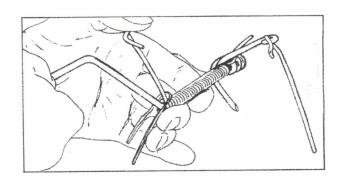
2. Now with the jaws in open position (as shown above) hook short curved end of tail over top of left jaw, which will cause the long end of the tail to be under the left jaw and on top of the spring.
