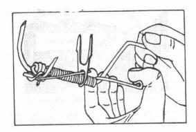
5. Move flat metal trigger to the end of the tail, (as shown above). Trap is now ready to use. ALWAYS **WEAR GLOVES WHEN SETTING THE** TRAP.
