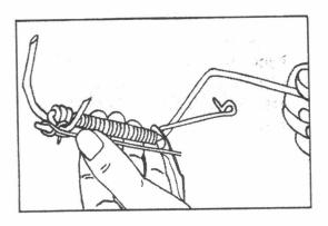
3. Slide flat metal trigger piece toward jaws with the points up. Put long end of the tail that is resting on the spring through the hole of flat metal trigger.
